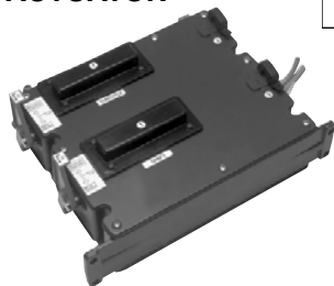
ECU (ELECTRONIC CONTROL UNIT)
